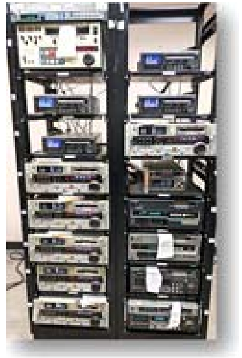
The equipment rack: 16 machines of various formats, transferring 16 hours of video to digital every hour.
